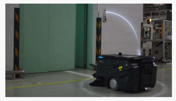
The PUDU MT1 integrates with IoT devices, interacting with elevators, gates, and other infrastructure for multi-floor cleaning. Remote monitoring via apps and PC interfaces provides real-time updates, visualized cleaning reports, and notifications when the trash is full, ensuring efficient management.
